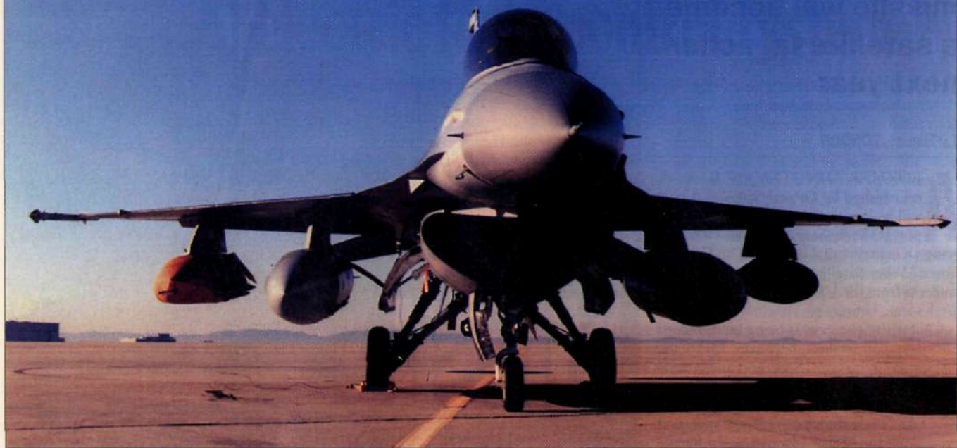
Advanced weaponry is becoming available on the F-16, including Lockheed Martin's Joint Air-to-Surface Standoff Missile (under outboard wing, left)
