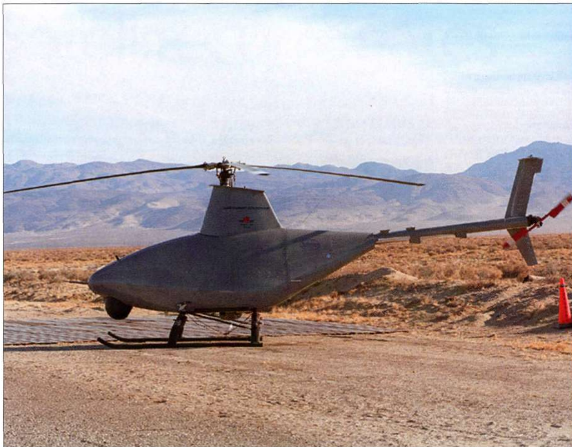
To minimise risk, Northrop Grumman's Fire Scout vertical take-off and landing tactical UAV, under development for the US Navy, is built around Schweizer's proven Model 330 light helicopter
