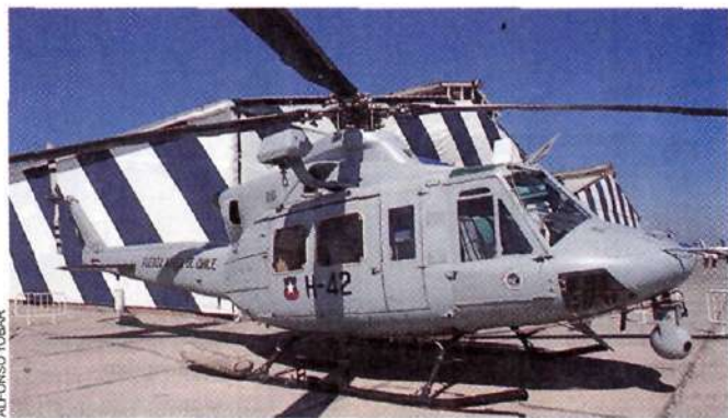
A Chilean air force Bell 412 has been equipped with the IAI HMOSP turret
