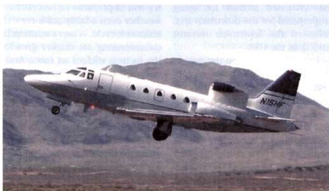
EJ22 takes off on Sabreliner testbed: the Eclipse is due to fly next month
