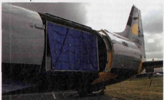
West Air has developed the ATP's large cargo door with BAe Systems
