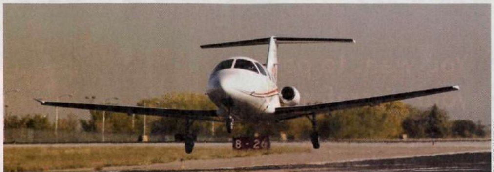
Flaps remained up and gear down during the first flight from Albuquerque, New Mexico, which lasted for 62min
