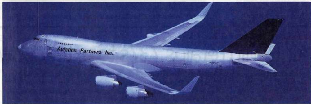
The winglet for the 747-400 was tested on a 747-200 proof-of-concept flight in 2000
