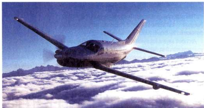
The TBM 700C2 offers an increased maximum take-off weight
