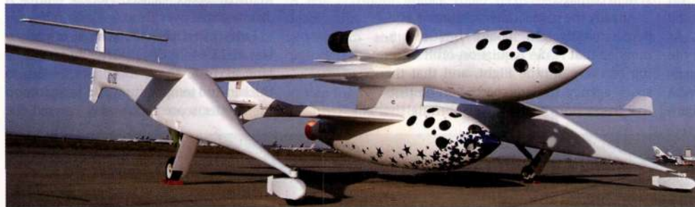
SpaceShipOne uses a specially developed hybrid rocket motor that burns NO 2 and HTPB
