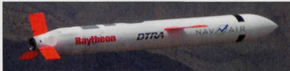
Initial production of 192 Block IV Tactical Tomahawks is under way, with first missiles due to enter service in 2004
