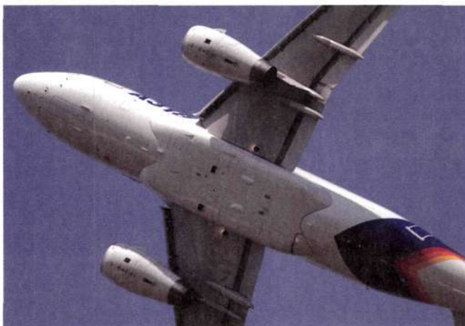
The 5-stage PW6000 accrued 350h of flight testing on the A318 with Airbus
