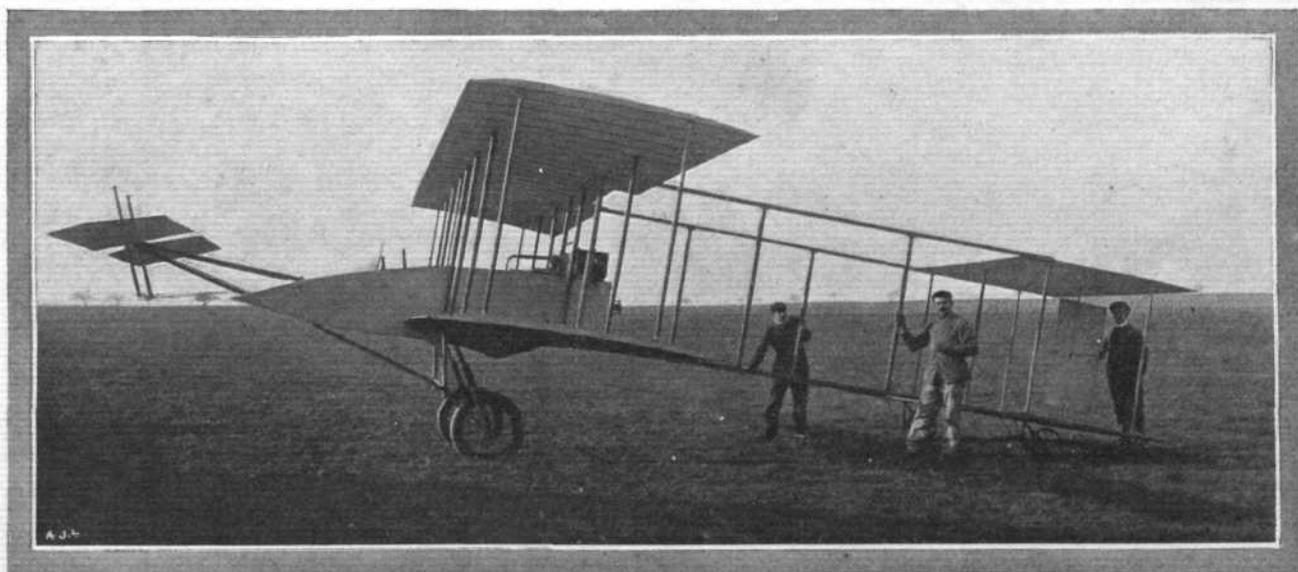
THE MAURICE FARMAN AEROPLANE.—Side view showing the double decks, the elevator in front, and the single rudder between the double-deck tail behind. The spread of the main wings is 10 metres, and the total weight 450 kilogs. The engine at present installed is a 50-60-h.p. Renault. The propeller is not shown.
