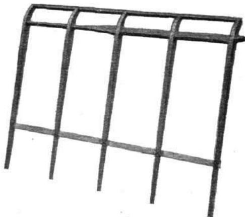
View showing a portion of the skeleton framework of the elevator on the Macfie monoplane.
