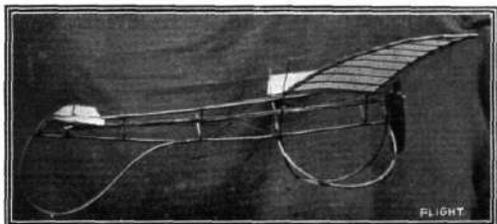
span over front plane, 22 ins.; length of one front wing,  $6\frac{1}{2}$  ins.; greatest chord of front wing, 44 ins.; 12 in. propeller of 25 in. pitch; total supporting surface, 284 sq. ins.; total weight with 22 strands of  $\frac{1}{16}$ -in. strip elastic,  $10\frac{1}{2}$  ozs.
