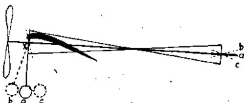
model is flying. Should the model's head be thrown down, the pendulum will be at *b*, should the tail fall, at *c*, and in horizontal flying at *a*. The movement of the pendulum will, of course, govern the tail, which at *a*, *b* and *c* corresponds with the *a*, *b* and *c* of the pendulum.
