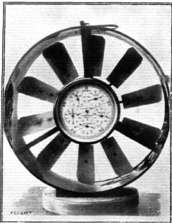
A windmill type of anemometer.
