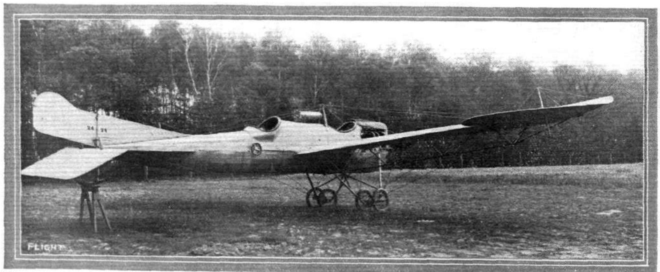
Three-quarter rear view of a D.F.W. monoplane, school type. It will be noticed that this machine is almost exactly similar to the military type, except for the steel bridge girder underneath the wings.
