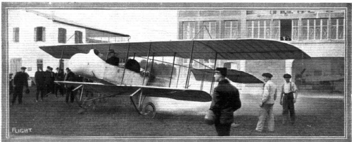
THE BLÉRIOT BIPLANE.—Amongst the Blériot machines which will be exhibited at the coming Paris Salon, is a biplane of the type shown in the accompanying photograph. This machine is constructed of steel throughout and has, it will be noticed, a new type of landing chassis which is said to be very effective even on the roughest ground.
