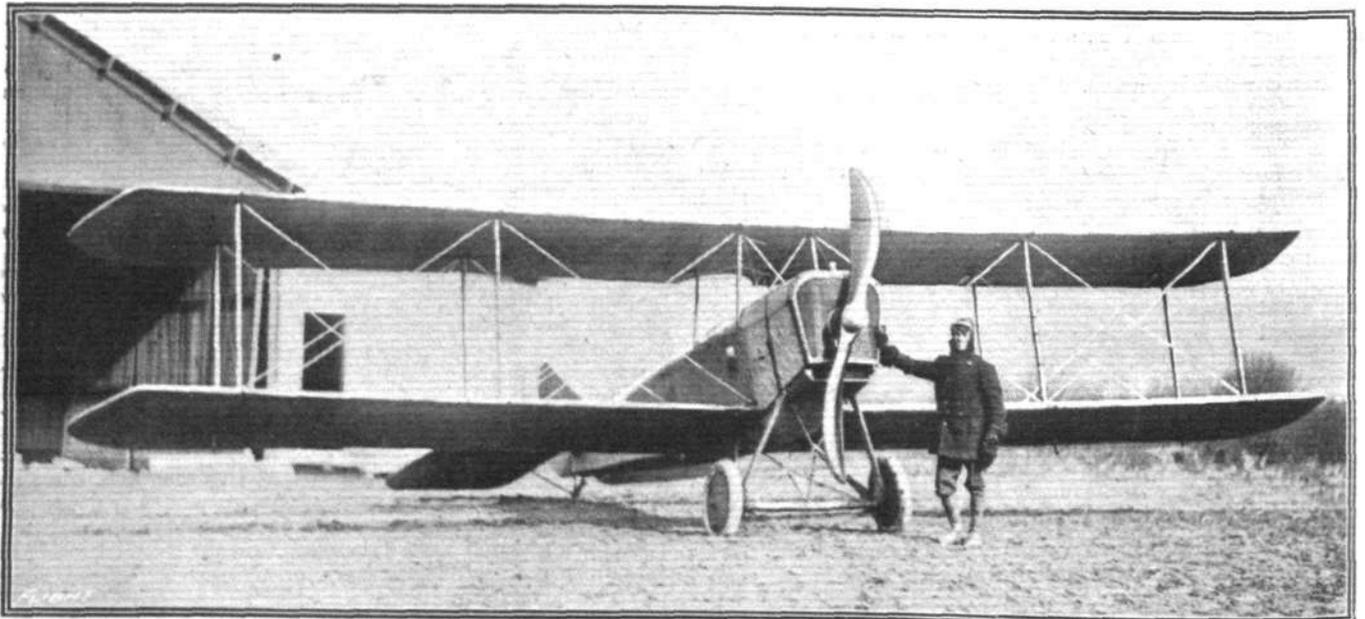
THE NEW THOMAS MILITARY TRACTOR BIPLANE, TYPE D2.—Fitted with one of the new 135 h.p. Thomas aeromotors, this machine is said to have attained a speed of 102 m.p.h., which constitutes, it is claimed, an American record.
