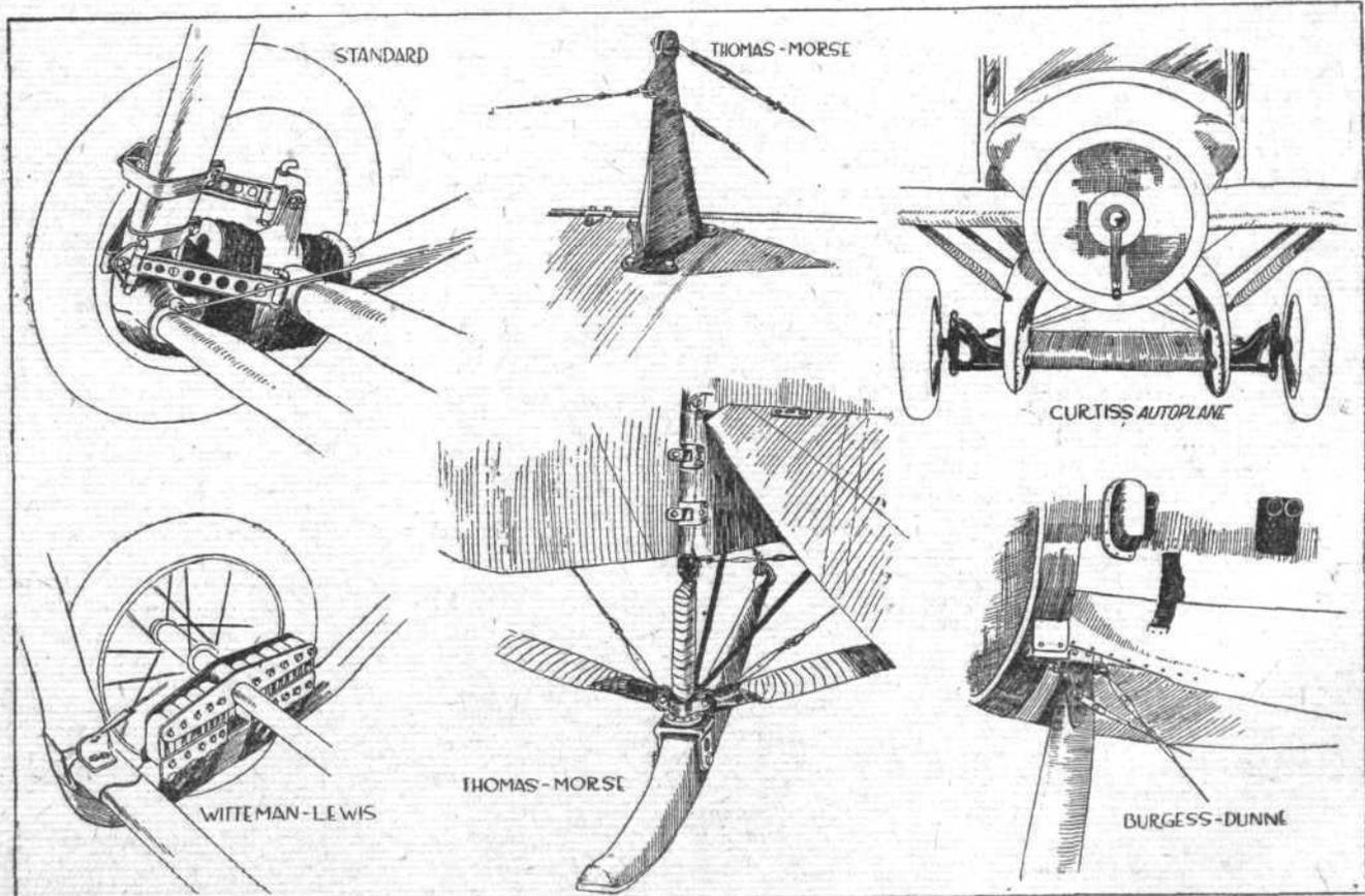
AT THE AMERICAN AERO SHOW.—Some constructional details. From left to right, top row: The shock-absorbing device on the chassis of the Standard tractor; control-surface crank-lever on the Thomas tractor; the front steerable wheels on the Curtiss "Autoplane." Bottom row: The Wittman-Lewis bridge-type shock-absorber; tail-skid on the Thomas tractor; the rear strut attachment to the nacelle of the Burgess-Dunne seaplane.
