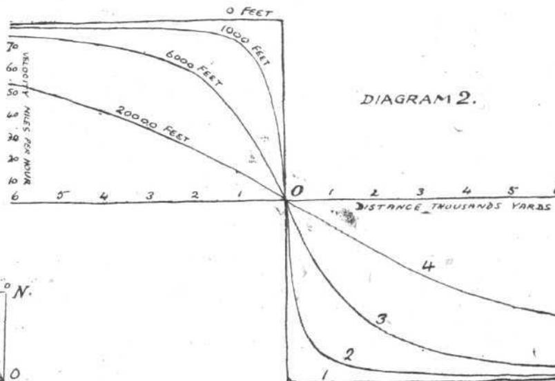
flying below 6,000 ft.—the fall of the note will be most marked when the plane is within 2,000 yards of the observer. In conclusion it is insisted, that only when the actual velocity of the plane through the air is rapidly increasing, and the plane is diving along the line of sight, could the note ever be heard to rise.
