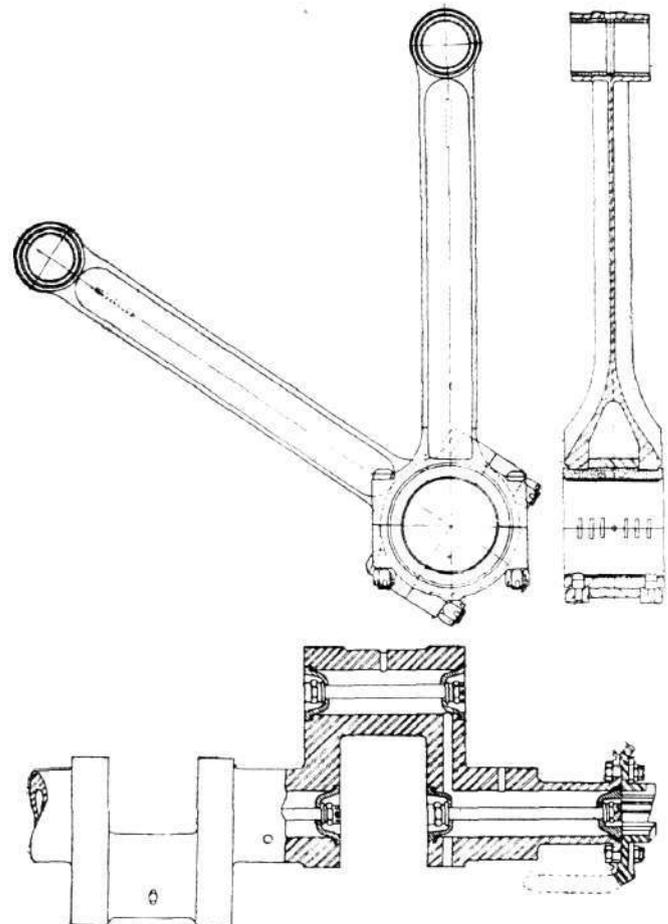
**Liberty con. rod assembly in side view and section. Bottom: Detail of crankshaft, showing method of plugging bores.**
