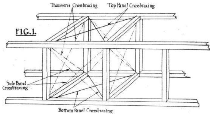
Each of these panels in the side of the fuselage helps to take bending moments in an upward or downward direction, while the corresponding panels in the top and bottom enable the structure to stand up to side loads of a similar nature.
