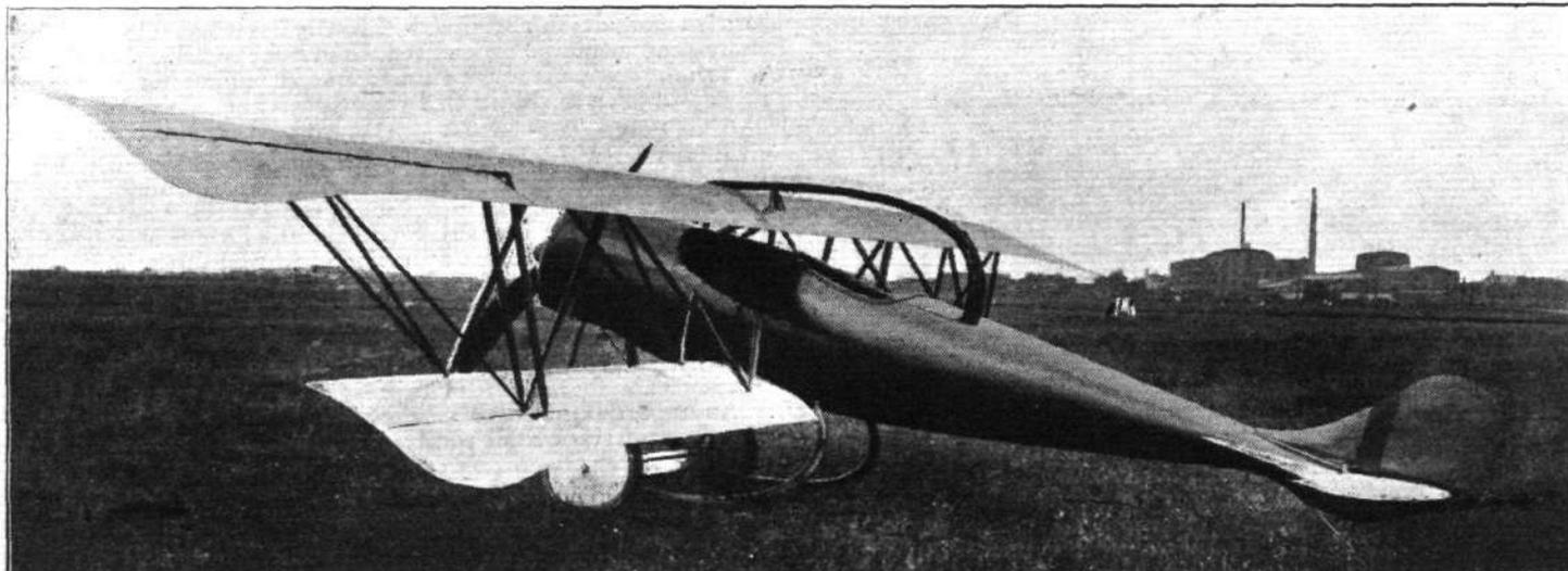
**THE DIMINUTIVE BIPLANE RECENTLY CONSTRUCTED AT THE PAALSON FACTORY IN SWEDEN:** It weighs 700 lb., and carries 400 lbs. at 80 m.p.h. with a 50 h.p. Thulin-Gnome engine. Note the strutting and the peculiar "gadget" above the body—presumably a sort of hand-grip for picking up the machine and carrying it home!
