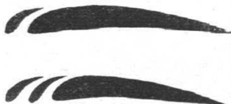
The Handley Page Wing: Diagram showing single and double slot arrangement
