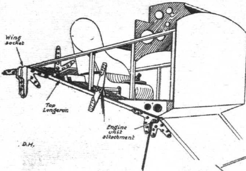
**THE D.H. 29 MONOPLANE :** The Pilot's Cockpit is placed above the top of the Fuselage and just in front of the Wings.
