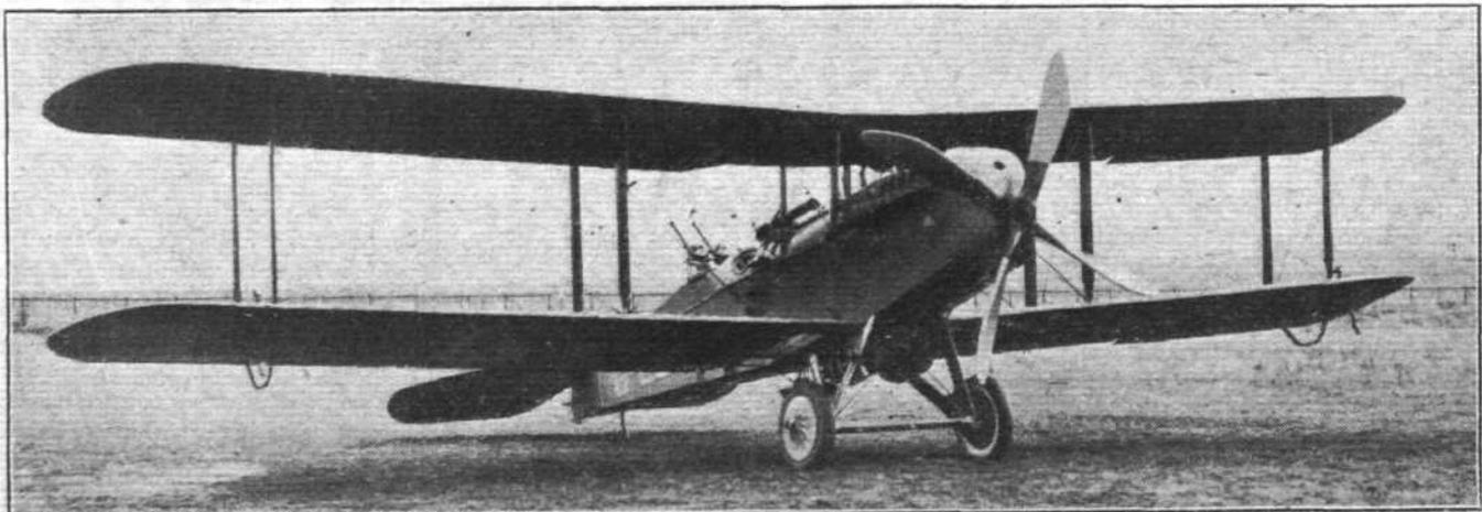
**An A.D.C. Modification :** This D.H.9 has been altered considerably by the Aircraft Disposal Company, and among other changes will be observed the substitution of Lamblin radiators for the usual nose radiators.
