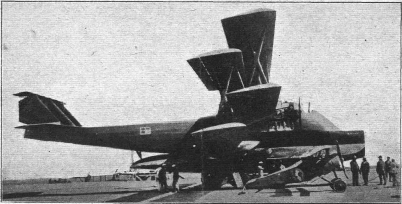
**THE BESSON H5 QUADRUPLANE FLYING BOAT :** Side view, in which an idea of its proportions may be obtained by comparison with the figures and the Nieuport machine in the foreground.
