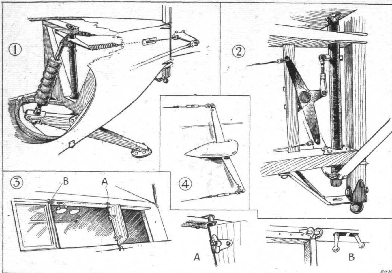
**THE D.H.50—SOME CONSTRUCTIONAL DETAILS:** 1 shows the steerable tail skid, with its rubber compression block springing. In 2 are shown the details of the tail trimming gear. 3 shows the deflector mounted outside the open starboard window. 4 streamline fairing over end of elevator layshaft.
