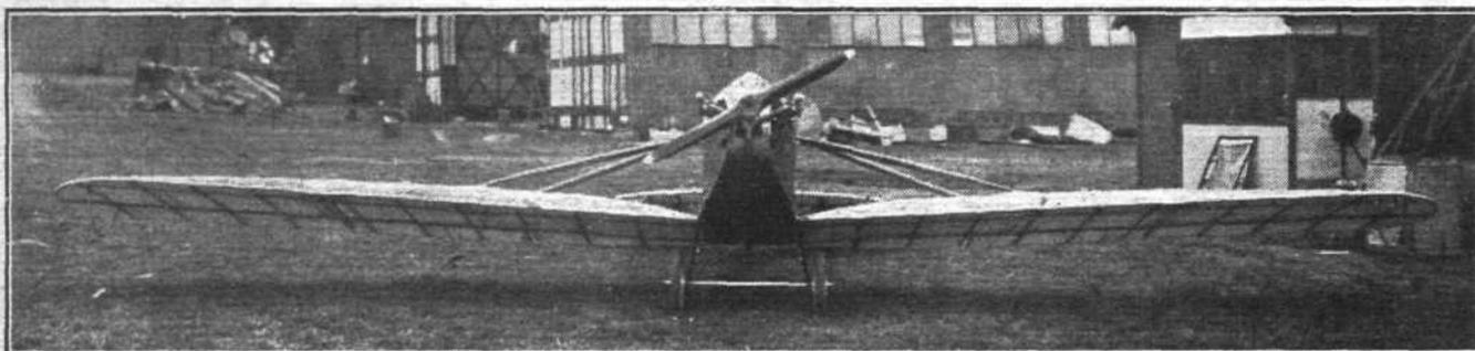
THE D.H. 53 : Front view, showing dihedral, wing bracing, struts, etc.
