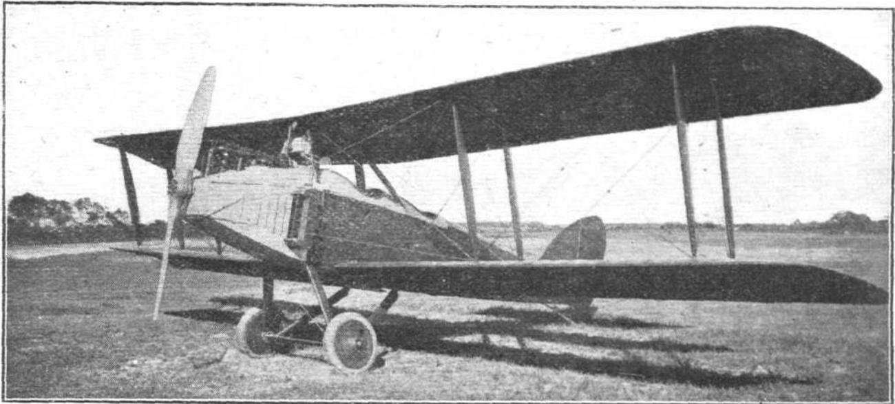
**A CHINESE-BUILT AEROPLANE:** A three-quarter front view of the "Schoettler I" biplane, fitted with a 160 h.p. Mercedes engine. This machine was built and flown at the Lunghwa Aerodrome, China, during the summer of this year.
