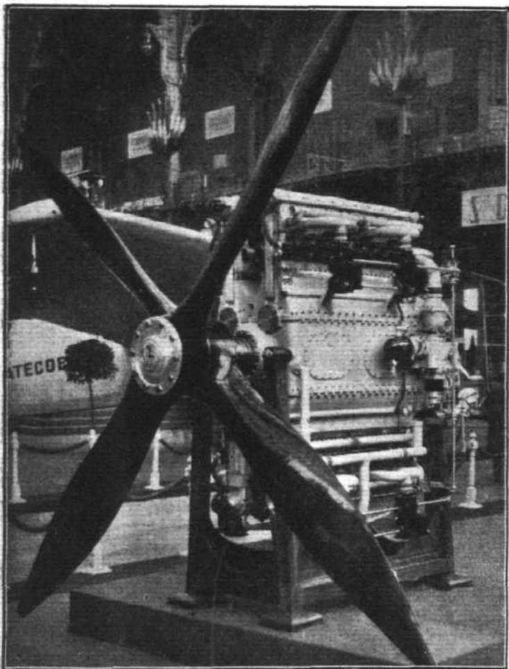
**THE BIGGEST AERO ENGINE AT THE SHOW :** This is the 1,000 h.p. Breguet aero engine, which consists of two Breguet-Bugattis placed on opposite sides of a common crankcase. The engine would be somewhat difficult to instal in an aeroplane of ordinary size.
