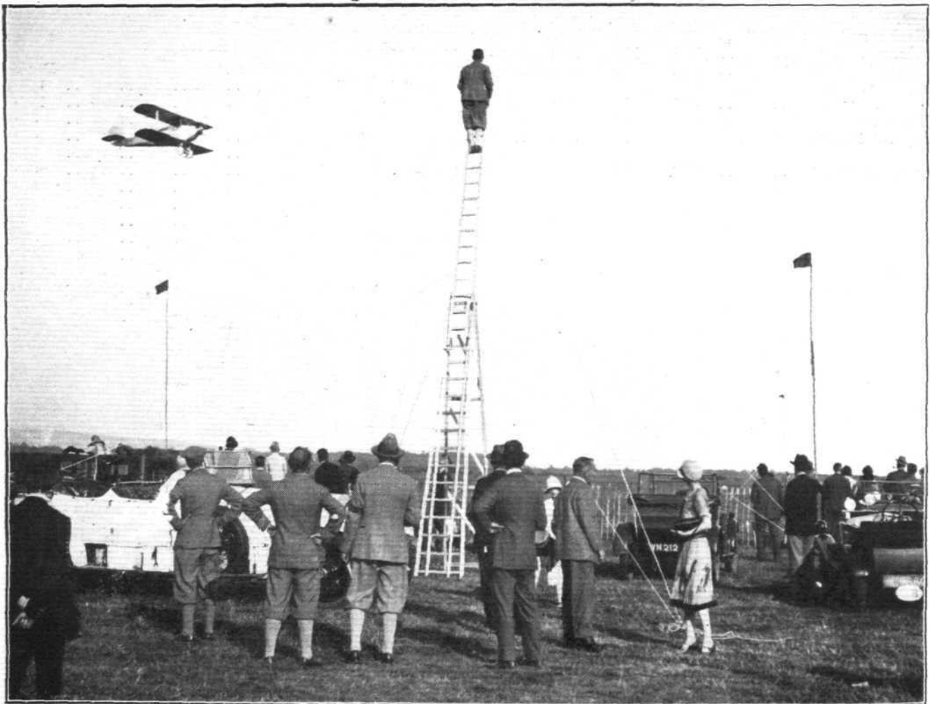
["FLIGHT" Photograph "OVER THE STICKS": This photograph gives a good idea of the manner in which the take-off tests were observed. On the ladder is Major Buchanan, of the Air Ministry, while among those in the foreground may (or may not) be recognised Major Mayo, Lieut.-Col. Sir Francis McClean, and Mr. C. C. Walker. The machine "going over the top" is the Blackburn "Bluebird," piloted by Squadron-Leader Longton.
