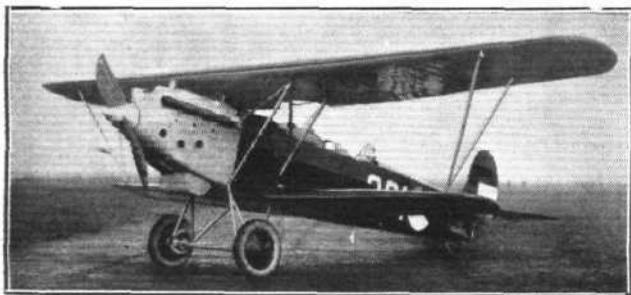
**THE FOKKER C. V. can be supplied with a number of different engines, and can be quickly converted into a two-seater fighter, a reconnaissance machine, a bomber, or even a school machine.**
