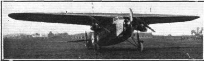
**THE FOKKER F. VII. 3m is a commercial monoplane. The three engines fitted are Armstrong-Siddeley "Lynx" of 180 h.p. each.**
