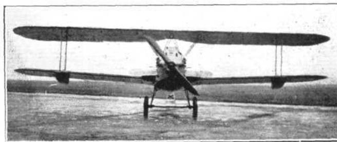
**The P. Levasseur three-seater naval reconnaissance aeroplane has a detachable undercarriage and a water-tight fuselage.**
