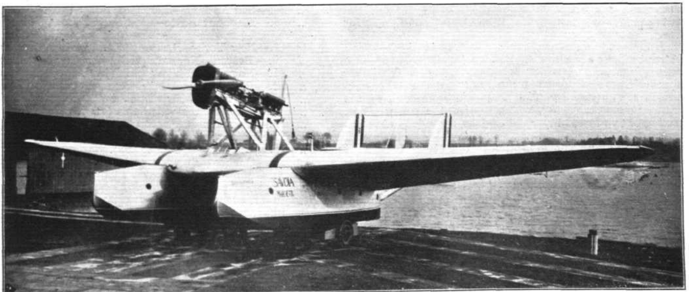
PINEDO'S BIG FLIGHT : The Savoia S.55 mono-seaplane, fitted with two 500 h.p. Isotta-Fraschini engines. Above, Col. The Marchese di Pinedo, the famous Italian pilot who just completed his 25,000-mile tour, involving two Atlantic crossings.
