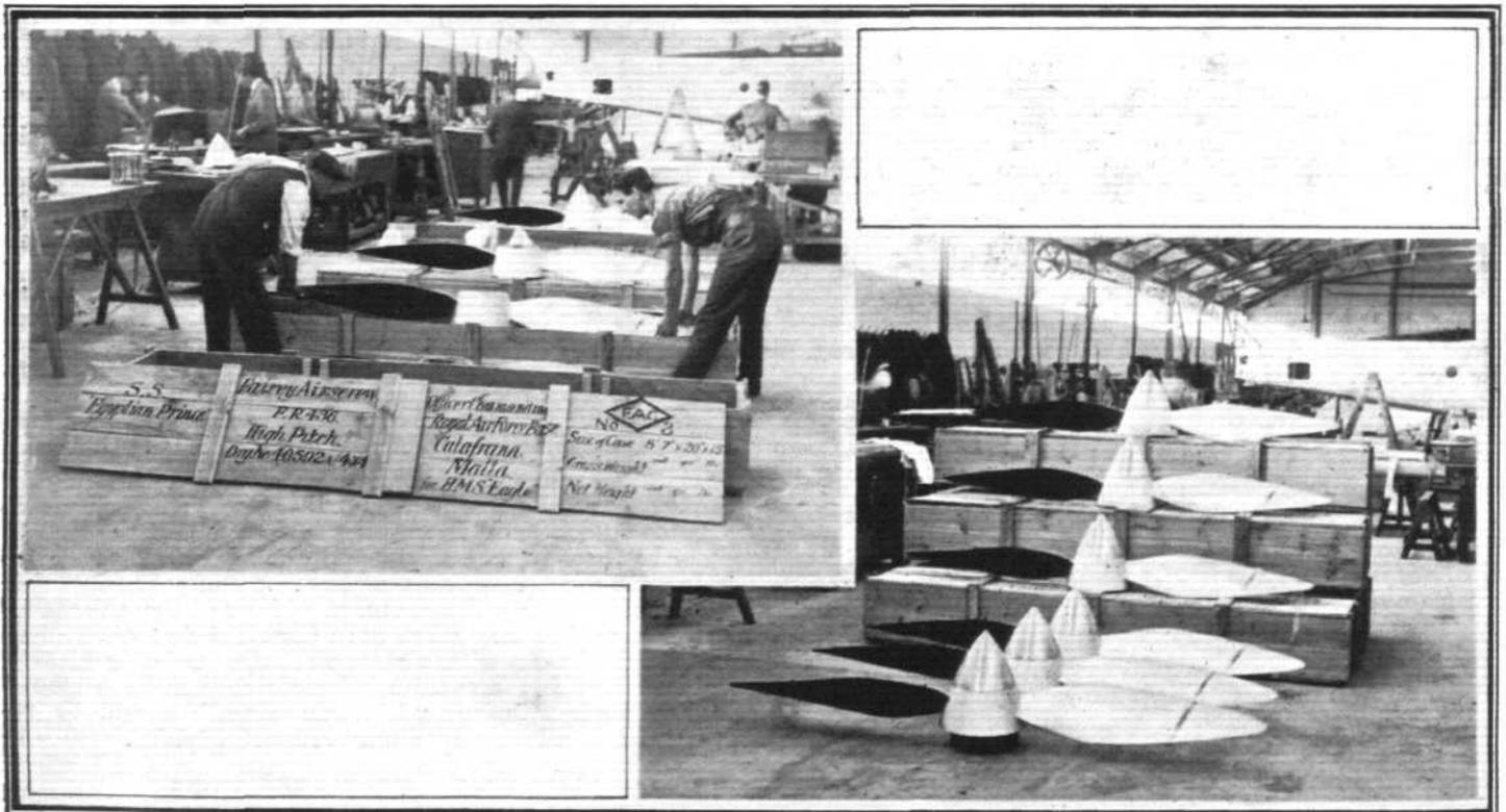
FOR THE SCHNEIDER TROPHY RACE: A batch of Fairey-Reed metal airscrews being packed for transport to the Mediterranean. In the right-hand photograph six of these propellers are seen, with their packing cases. The pitch of the blades makes it quite evident that the propellers are for high-speed machines.
