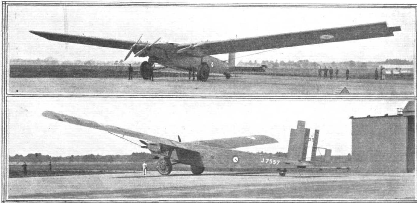
**THE BEARDMORE "INFLEXIBLE"**: With a wing span of 158 ft., and a total loaded weight of about 15 tons, this machine is an interesting experiment in beating the scale law. Three-quarter front and three-quarter rear views.
