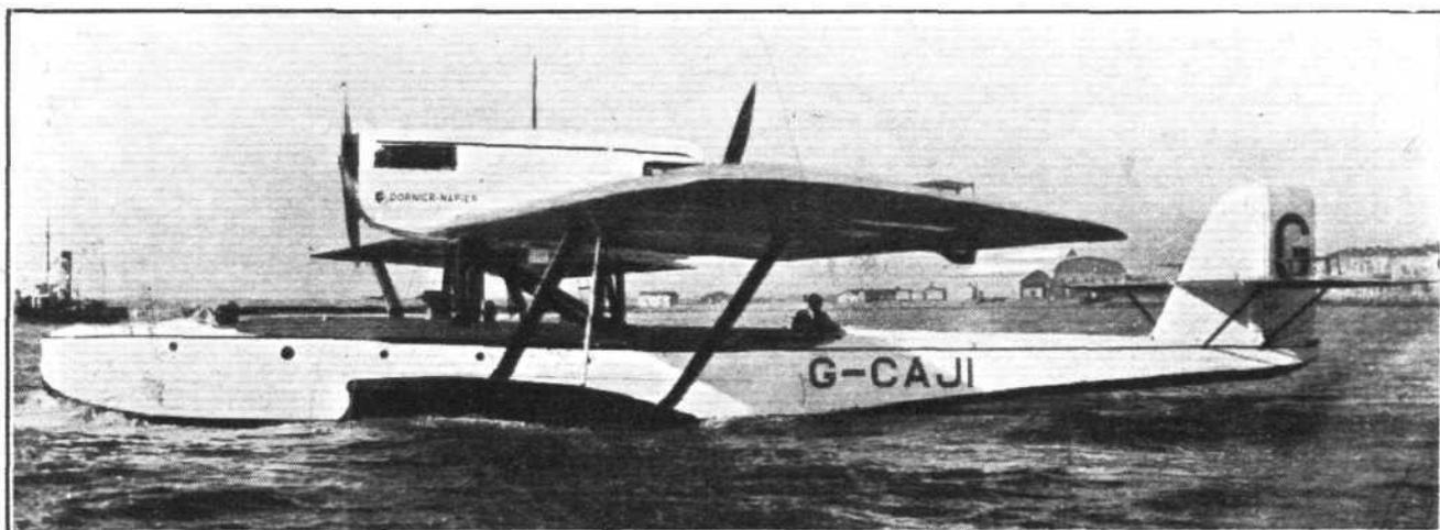
**FOR THE ATLANTIC FLIGHT:** The Dornier-Napier all-metal flying-boat, fitted with two 450 h.p. Napier "Lion" engines, in which Capt. F. T. Courtney is attempting a return flight across the Atlantic. It is equipped with Marconi wireless.
