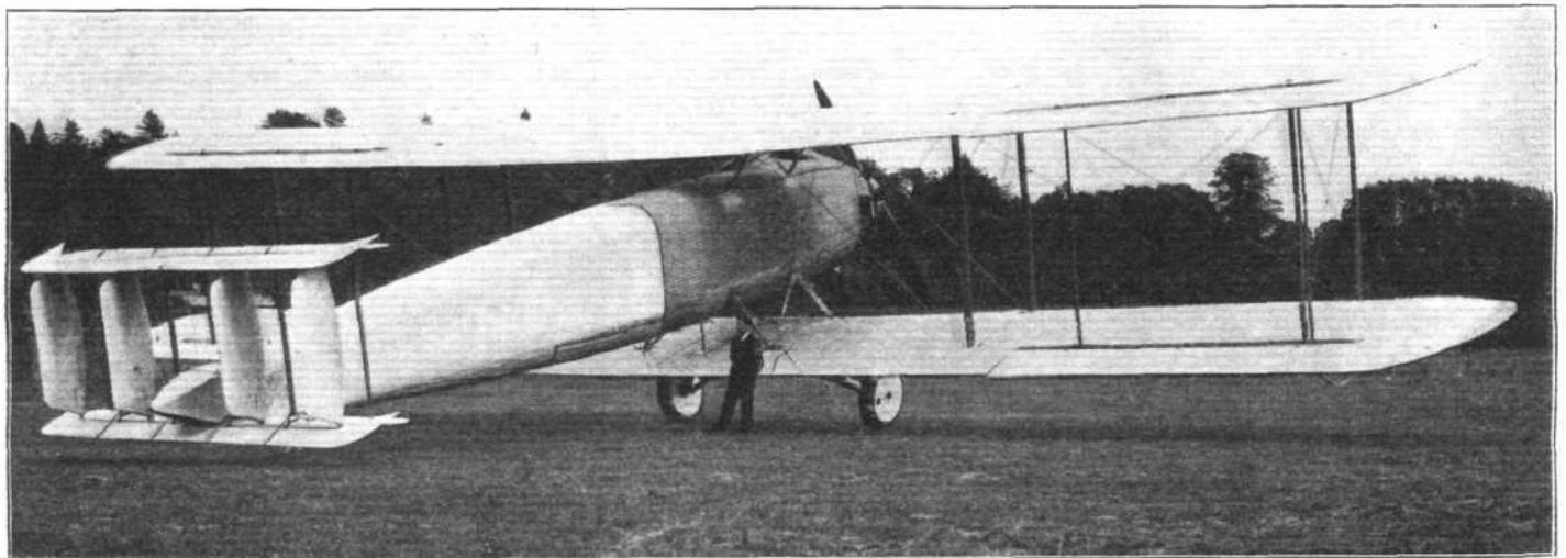
**THE VICKERS "VELLORE" FREIGHT CARRIER : Three-quarter rear view. Note the biplane tail and the four rudders. The man standing next to the machine gives a good idea of the size.**
