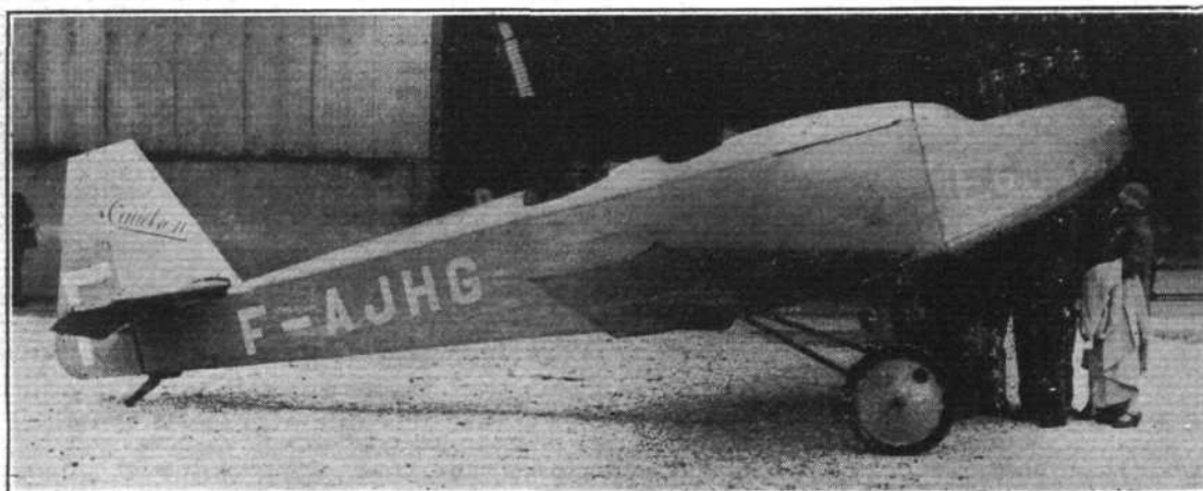
The latest Caudron type 193 low-wing monoplane (85 h.p. Renault). ("FLIGHT" Photo.)
