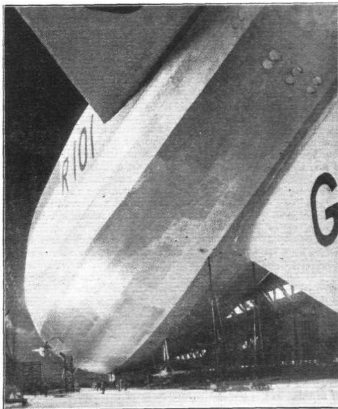
In this view from under the tail of R.101 the aft openings of the internal air pressure system are clearly seen. (“FLIGHT” Photo.)
