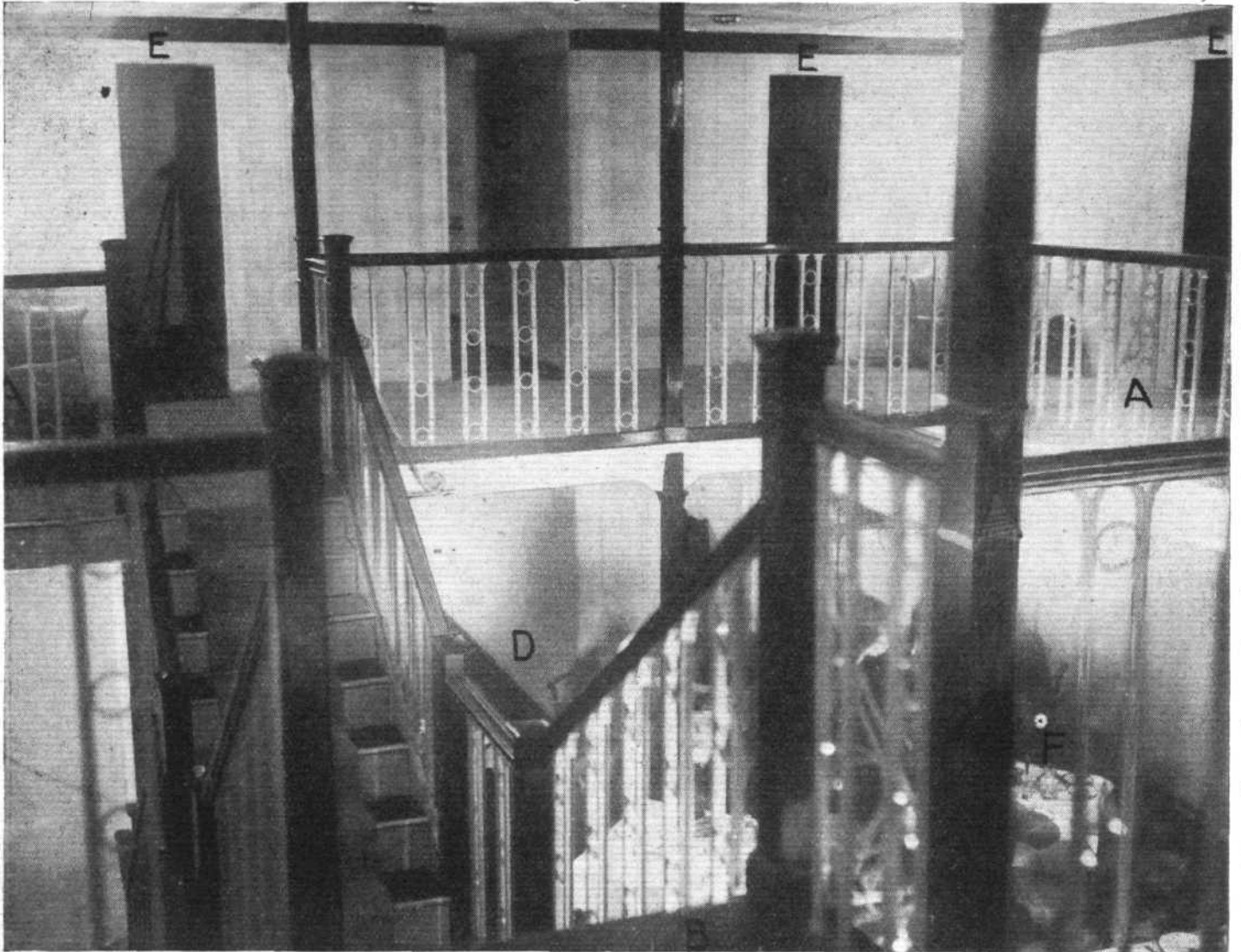
On the gallery or top deck. The saloon is below. A A : The gallery. B : Double staircase down to saloon. C : Passage to upper balcony. D : Passage to lower balcony. E E E : Entrance to cabins. There are similar cabins on the second deck. F : Passengers at lunch table in saloon. (FLIGHT Photo.)
