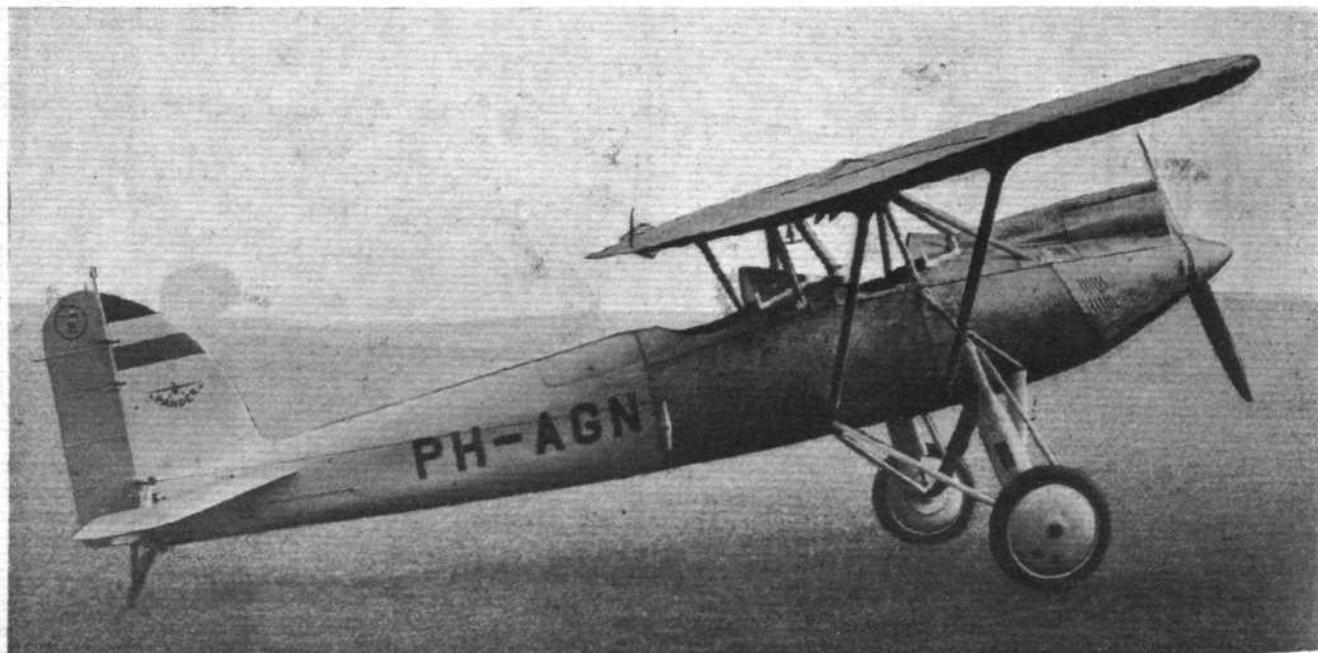
**THE PANDER-GIPSY :** A Dutch private owner's machine, which, fitted with the D.H. Gipsy engine, has a top speed of 125 m.p.h. and a landing speed of 50 m.p.h. This machine is fitted with Bendix wheel brakes as standard.
