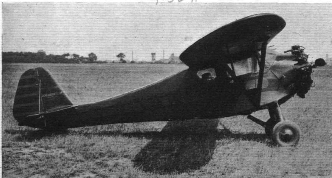
FOR THE INTERNATIONAL TOURING COMPETITION: The American "Monocoupe" Special with Warner "Scarab" engine, has been entered by Mr. Trench, and is to be piloted by Mr. Carberry. The machine has side-by-side seating. The wheels are Goodrich, and brakes are fitted.
