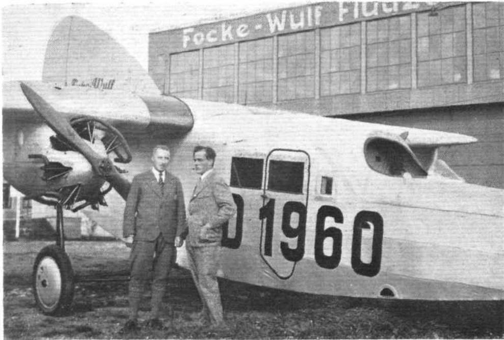
THE FOCKE-WULF "ENTE": Note the pilot's cockpit, the cabin door, and the petrol tanks in the wing. Standing by the machine are Herr Focke and the firm's chief test pilot, Herr Edzard.
