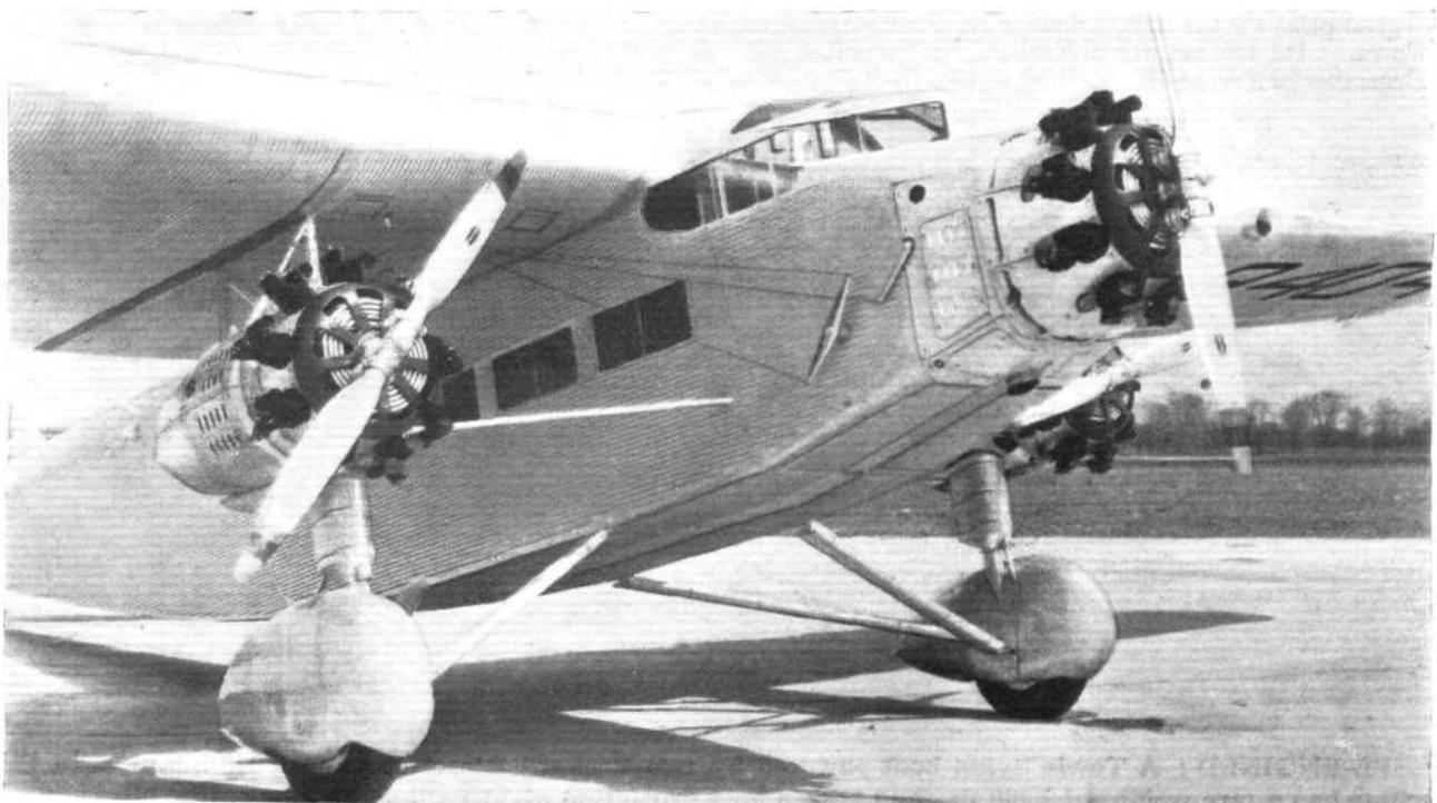
**DIESEL-ENGINED :** A Ford type 4-AT, fitted with three Packard Diesel engines of 225 b.h.p. each. With these engines the machine has a cruising speed of 100 m.p.h. It carries two pilots and 11 passengers.
