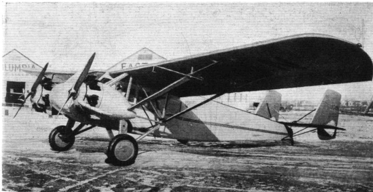
The Curtiss "Kingbird": An American 8-place twin-engined cabin monoplane, fitted with two 225 h.p. Wright "Whirlwind" engines.
