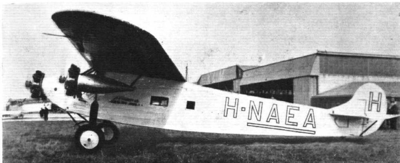
Above is shown the Fokker F.VIIb, fitted with three Armstrong-Siddeley "Lynx," or Gnome-Rhone "Titan" engines, one of the types used both by K.L.M. and K.N.I.L.M. Another type used on the Amsterdam-Batavia line is the Fokker F.IX (three Bristol "Jupiters") shown below. The centre picture is an aerial view of Aleppo, on the original route to Batavia.
