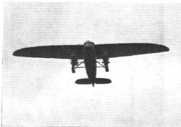
**THE DO K IN FLIGHT:** The projections behind the engines are the mudguards over the wheels.
