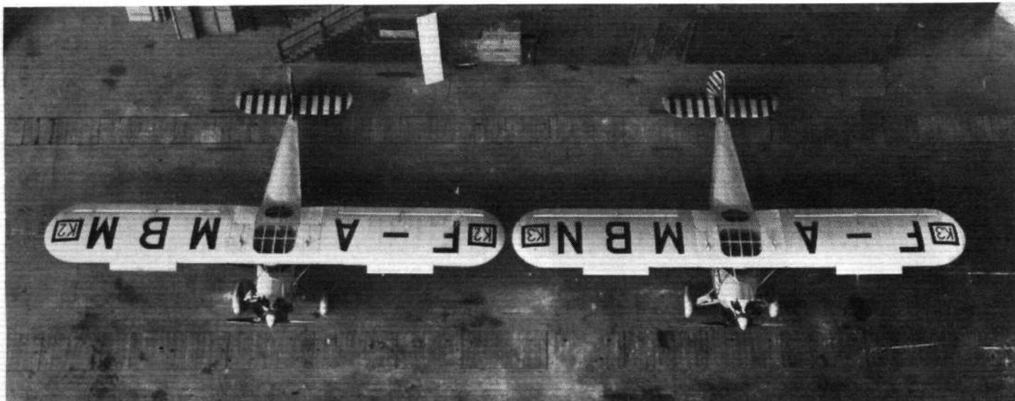
**TWO FRENCH COMPETITORS:** The Potez 43 machines are fitted with permanently-open slots.
